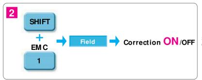
Set Correction to ON. The corrected data is reflected on the screen data.
